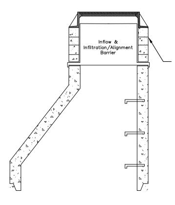
IF USING CONCRETE ADJUSTING RINGS AN ALIGNMENT OR INLFOW & INFILTRATION BARRIER MUST BE INSTALLED. I & I BARRIERS SHALL BE SEALED TO THE CONE USING THE PRODUCT APPROVED GROUT OR SEALANT. CONCRETE ADJUSTMENT RINGS SHALL BE SEALED TO THE CASTING, AND ONE ANOTHER BY USING A PREPACKAGED MOTOR MIX OR MFG SPECIFIED MIX FOR NON—CONCRETE RINGS. TOTAL ADJUSTMENT MINIMUM 4" MAX 14".
